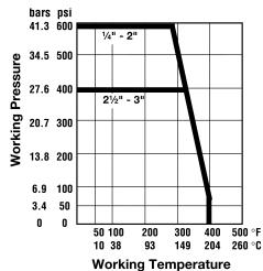
\*See applicable note on reverse side for solder end valves with regards to pressure/ temperature rating.
